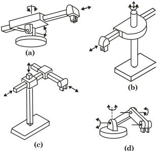
**Figure (i) (a):** Polar configuration uses a telescopic arm that can be raised or lowered about a horizontal pivot. The pivot is mounted on a rotating base. These various joints provide the robot with capacity to move its arm within a spherical space, and hence its name spherical coordinate robot.
